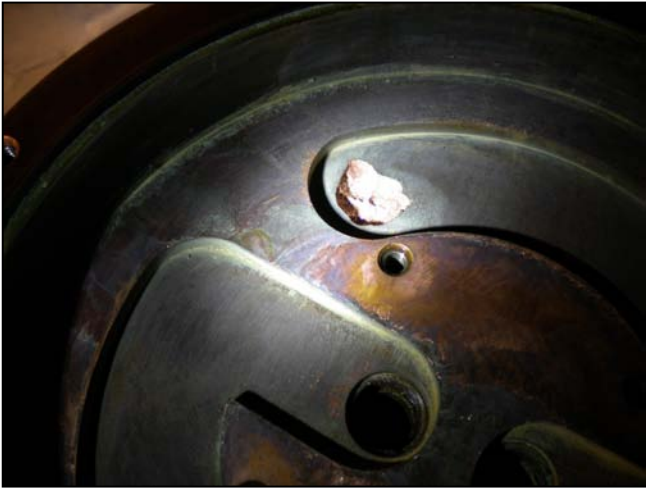
Physical erosion in copper cathode body caused by suspended particulates and/or air bubbles in cooling water system
