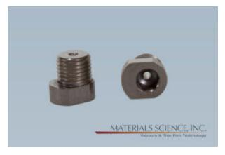
The cam screws have a high adhesion proprietary coating that adapts to cycling between atmosphere and vacuum without particulate generation or degradation that causes fretting wear. The coating will not wear off during use and operates reliably under all conditions the sputtering source will be exposed to. It is UHV compatible.
