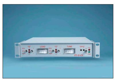
positive and negative error signals that the detector generates for driving the servo system should be virtually zero. The polarity of the error signal will determine the direction in which the servo motor will travel. This combined with the proper gain will ensure the proper tuning sequences.
