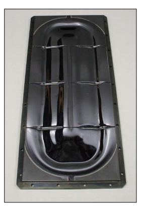
Eroded Tiled, Doped Silicon Target Bonded to Insert-Style Backing Plate
