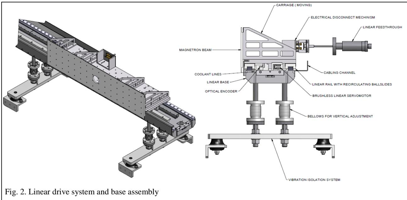
Fig. 2. Linear drive system and base assembly
