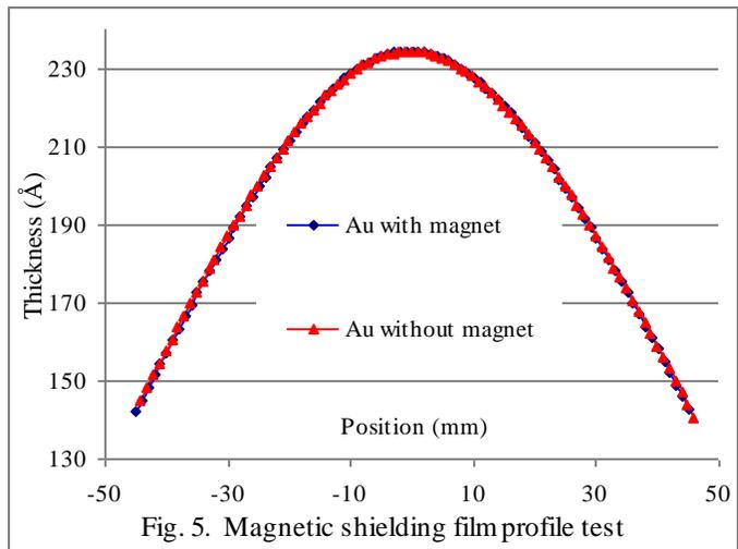
Fig. 5. Magnetic shielding film profile test
