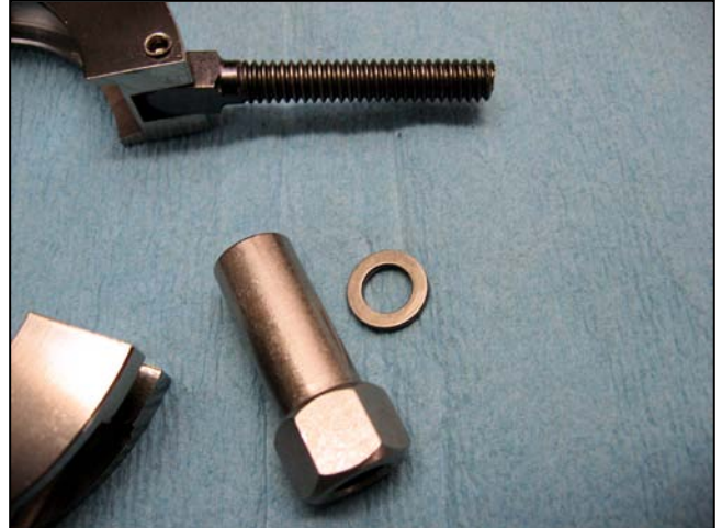
Adaptive i-Kote™ coating is applied to threads on KF-50 stainless steel swing clamp that is part of tilt mechanism. Screws on assembly also have the coating applied.
