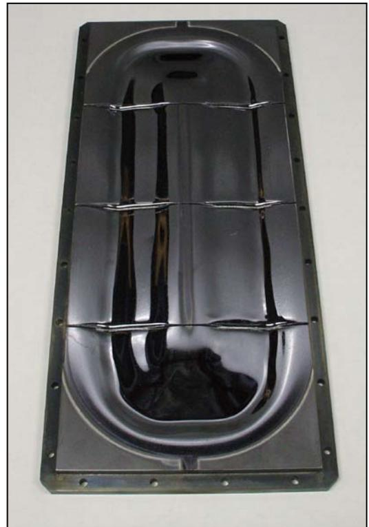
**Eroded Tiled, Doped Silicon Target
